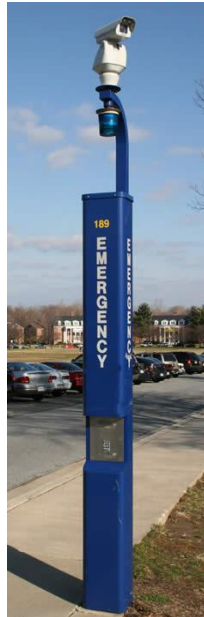
Figure 6: One of the surveillance cameras placed on the University of Maryland campus, capable of full tilt, 360°pan, and optical/digital zoom.
