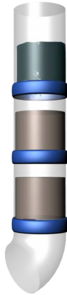
Figure 6.1 Diagram of water recycling column. The recycling column was constructed with a PVC column filled with layers of fine sand and gravel. Black gardening filters were placed between each layer, separating the sand and gravel. B. braunii algal solution entered the column from an opening at the top, and algae was filtered out as the solution passed down the column. Algae-free water exited through an outlet at the bottom of the column and returned to the CO 2 scrubbing column for reuse.
